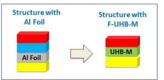
M helps Converting industry move from a 'difficult to recycle 4-ply laminate structure with aluminum foil' to a 'much simpler, easily recyclable 3-ply laminate structure with F-UHB-M film' without compromising on barrier performance, thus helping the customer achieve reduced laminate weight and lesser cost with minimized carbon footprint.
