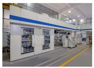
Combi Lamination Machine: UFlex's Combi Lamination Machine features a digital AC vector drive and
