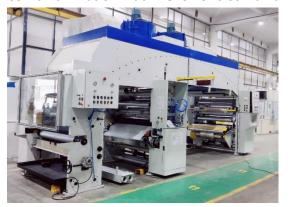
AC vector grade motor technology. This versatile model facilitates the lamination of two different substrates seamlessly using any of the two modes at a given time. The machine includes unwind and rewind features, a solvent-less coating unit, a gravure coating unit, a lamination unit, and a drying tunnel. With a speed of up to 300 meters/minute for solvent-based operations and 450 meters/minute for solvent-less operations, this machine sets new benchmarks in efficiency and performance.
